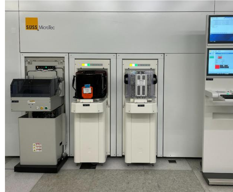
Suss MicroTec's 200/300 mm automated tool for debonding 2D materials (TMDCs) from a growth wafer.
