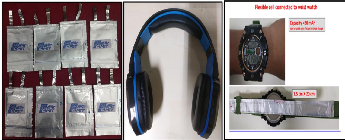
Flexible pouch type Li ion batteries and belt shaped Li-ion batteries for headphone and wrist watch developed by CMET
