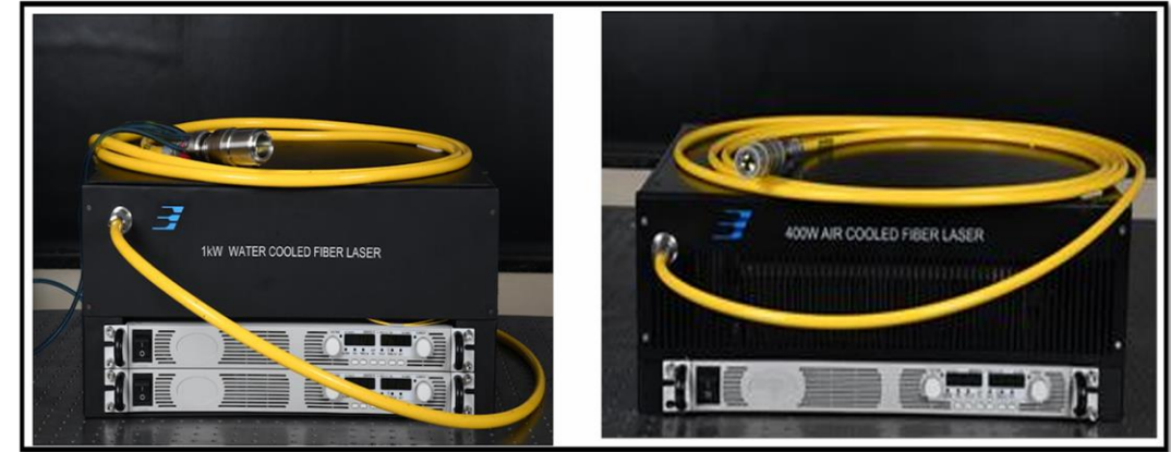
1kW water cooled and 400W air cooled Fiber Lasers developed under Nnetra project
