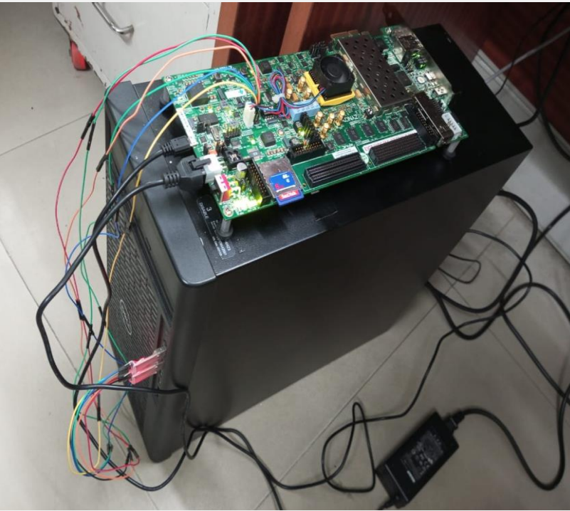
Znyq-zc706 FPGA board set up for AJIT IP implementation
