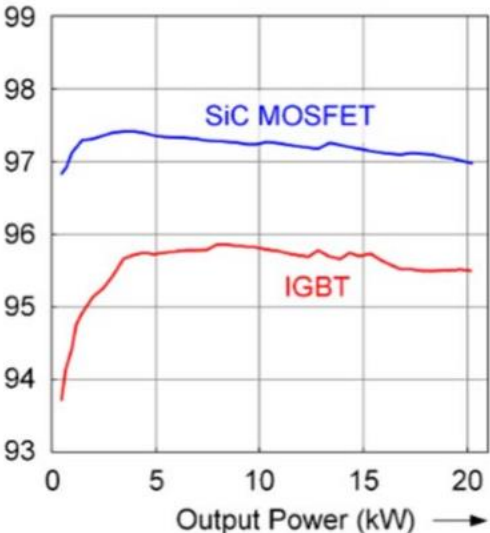
Fig. 2.3.1: Device efficiency in % vs. output power in kW [4].
