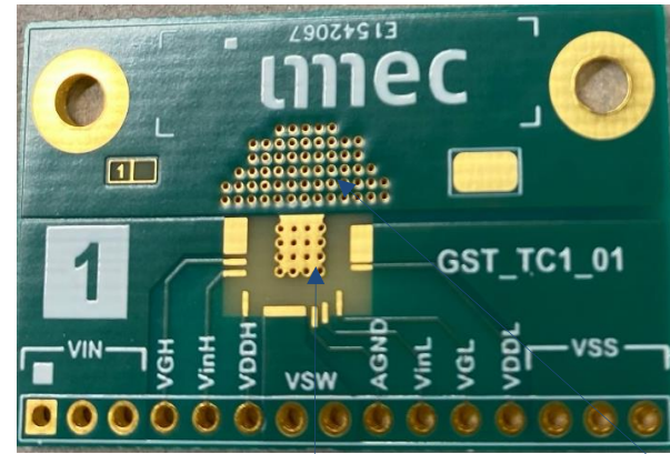
Thermal vias and metal on the back
