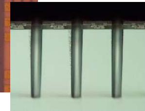
1. TSV blind via etch and isolation
