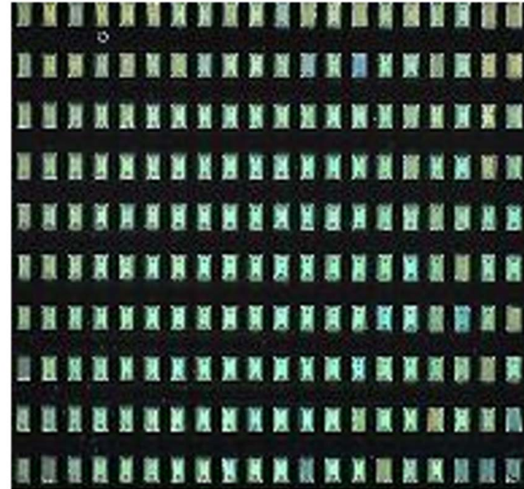
Self-Assembled Micro-LED chips (75 \mu m \times 125 \mu m)
