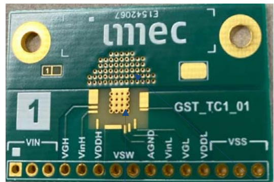
Thermal vias and metal on the back
