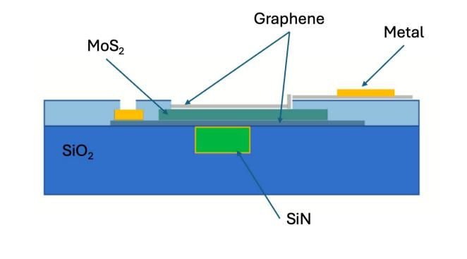
4. Memristors based on TMDs
