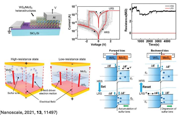
a) MIM structures, based on the formation and fusing of conductive filaments, suffer from serious structural damage of the 2D material  $\rightarrow$  low reliability, rapid failure
