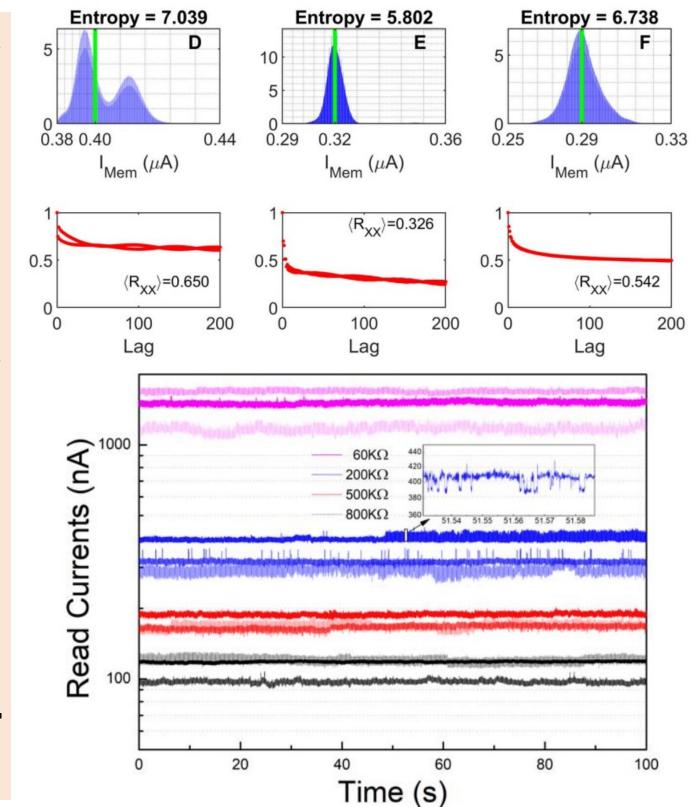
TRNG The Memristive SiNx circuit employs memristors to generate VREAD current noise signals. A comparator generates a bitstream based on a
