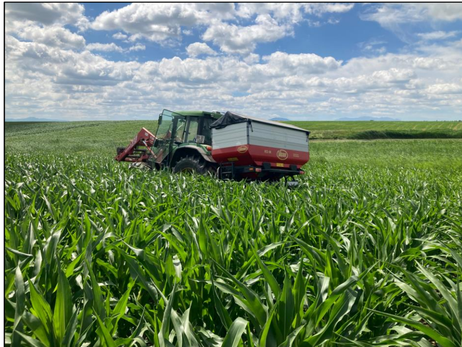
Urea spreading in-season with John Deere 6800 tractor and Vicon Geospread RO-M fertilizer machine driven and controlled with Trimble CFX GPS system
