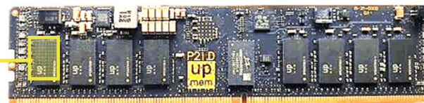
UPMEM PIM accelerator module
