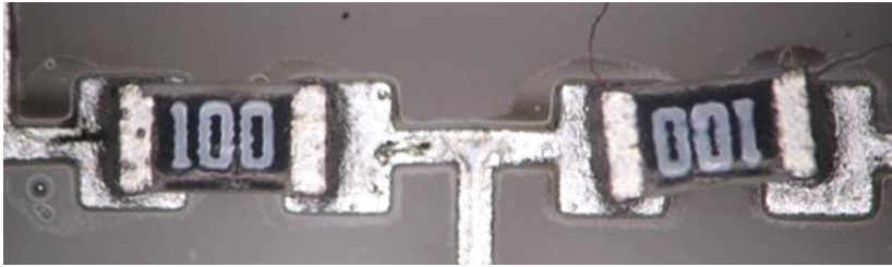
Test circuits made of PLA and CA materials Focus on low temp. Soldering.
